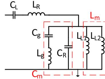
Fig. 4 The equivalent circuit of the proposed antenna.
