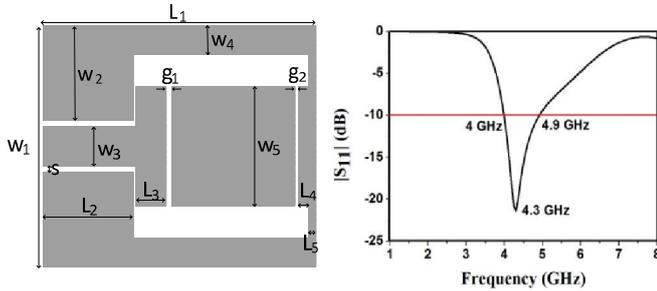
Fig. 2 (a) Dimensions. (b) Simulated return loss.
