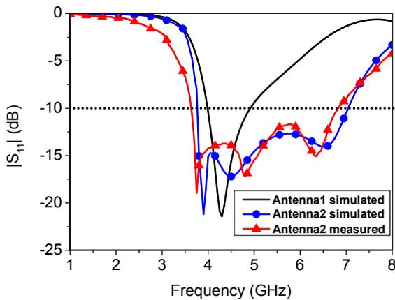
Fig. 5 Comparison of  $S_{11}$  between the two antennas.
