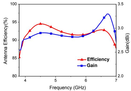
Fig. 6 Simulated gain and efficiency of the antenna
